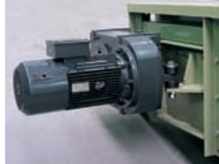
▲ Motor is equipped with a gear assembly (variable speed) mounted directly on the shaft, hung shock-proof on rubber 'silent blocks'.
