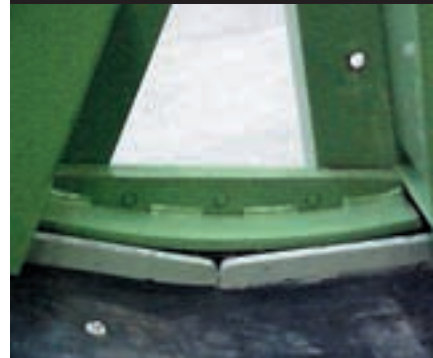
▲ Belt buckle with wear strips that can be changed (replaced) easily.
