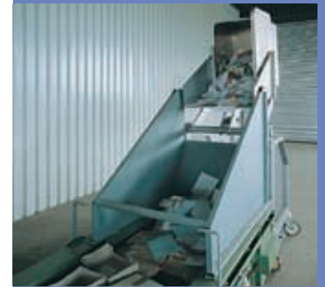
▲ Action principle of the optional container loading facility.
