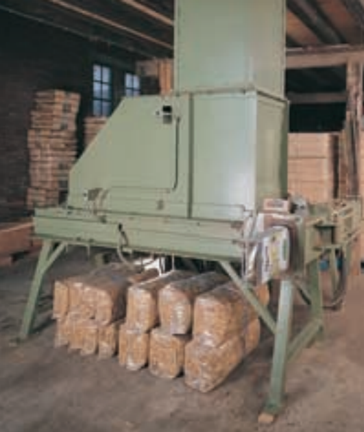
▲ The horizontal packaging press MAXIPACK HZP 200/240 PP (equipped with a pre-press flap).
