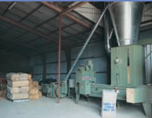
▲ The horizontal packaging press MAXIPACK HZP 300/500 - with volume switch - in action at a foraging company.
