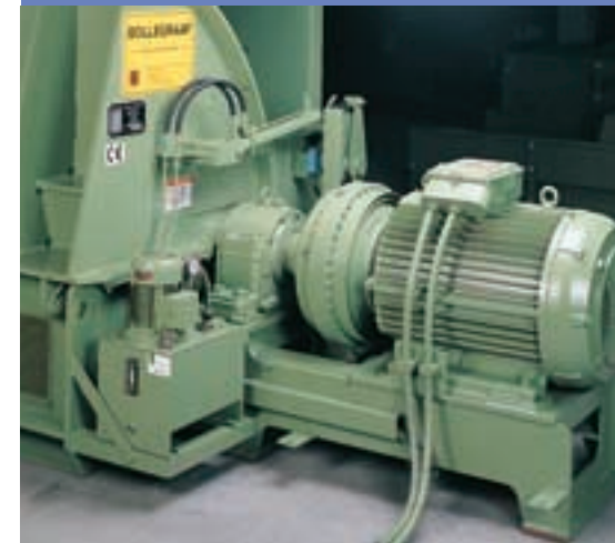
▲ 110 kW motor with oil coupling and roller bearing. The hydraulic bypass valve control on the shredder for passing the material without shredding.
