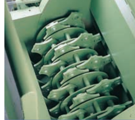
▲ Rotor with six-headed, replaceable hammers. The design ensures a very small particle size.
