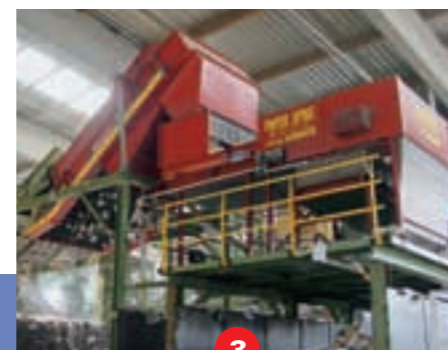
▲ Paper Spike® The Paper Spike® separates small pieces of OCC from paper.
