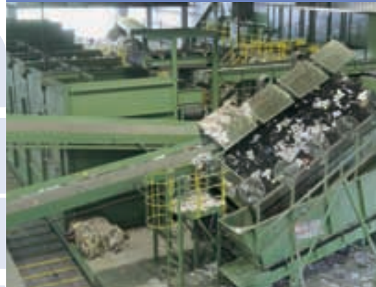
▲ Single Stream Installation RRA-York, USA. Capacity 20-22 tons per hour.
