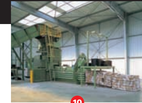
▲ Baler The baler processes the material up to homogeneous bales.
