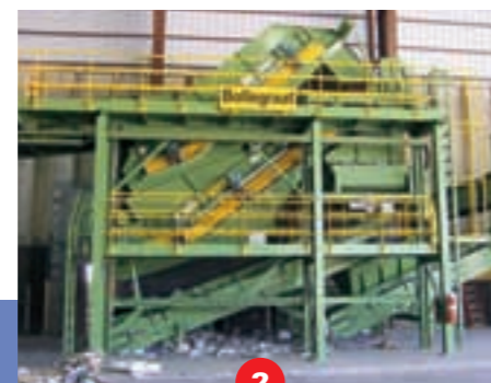
▲ Double ONP Screen Top deck of the screen separates newspaper from the single stream. Second deck contains a mix of newspaper and mixed paper. The throughput of the screen is mostly glass, bottles, cans and fines.
