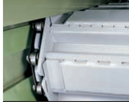
▲ The patented labyrinth sealing system prevents the chain from getting dirty.
