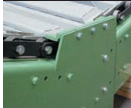
▲ Bend of the belt with wear strips that can be changed (replaced) easily.
